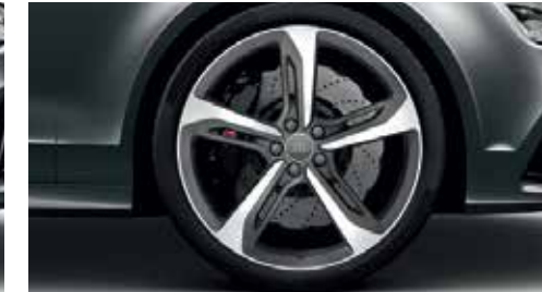
Cast aluminium wheels in 5-spoke blade design in matte titanium look, high-gloss turned finish size 9 J x 21 with 275/30 R 21 tyres*
