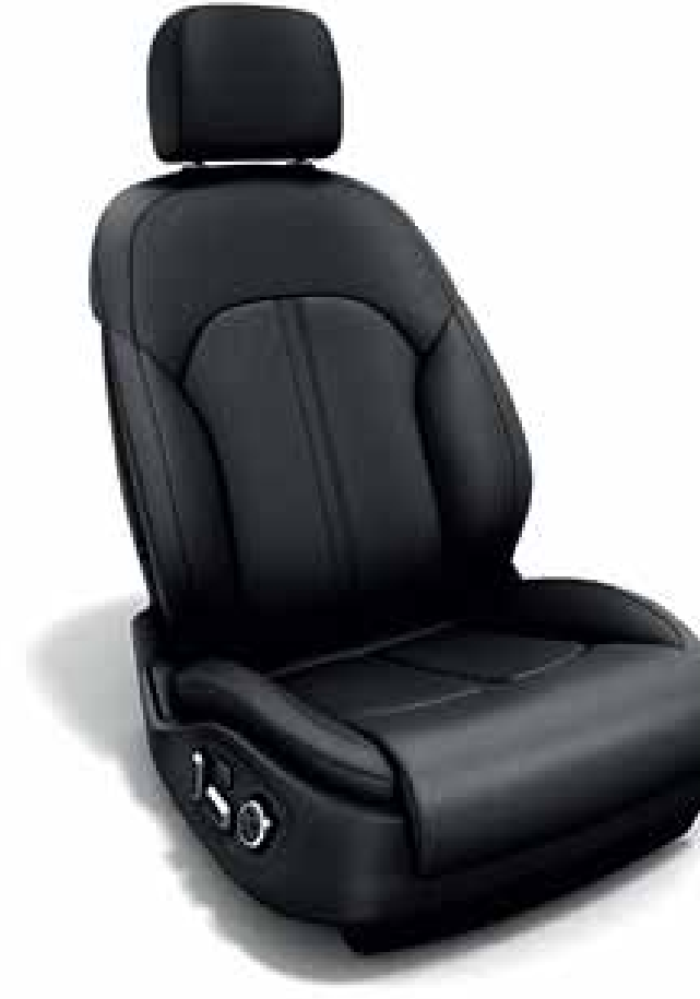
Comfort seats, front, with memory function* with electric adjustment of seat height, fore/aft position, backrest angle, seat angle and thigh support; pneumatic adjustment of seat and backrest side bolsters as well as lumbar support; manual adjustment of head restraint height and clearance, as well as seat belt height; including memory function for driver and front-passenger seat, electric steering wheel adjustment and exterior mirrors; optional seat ventilation, front (The image shows comfort seat, front, with memory function and seat ventilation, front, in perforated Valcona leather, black.)
